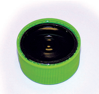
Baffle Fabricated from Bottle Cap
