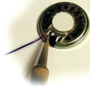
Figure 15 - Soldering to the Speaker Terminals
